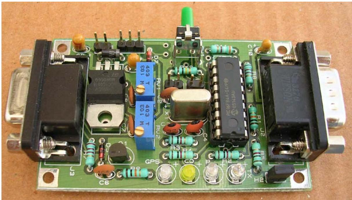
FoxTrak is designed on a Double Sided PTH Board Measuring 7 x 4.5cm
